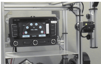
Optical Inspection System – each piece of screen content on the Infotainment System is photographed and verified.
